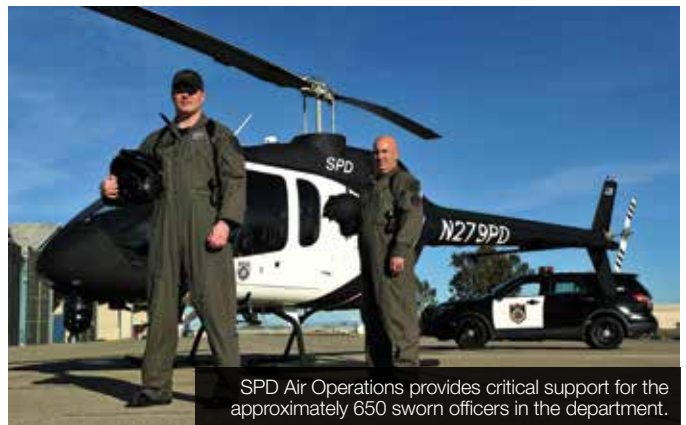
The new Bell 505 is equipped with a full suite of mission equipment, including the L3 Wescam MX-10 HD camera visible on the nose of the aircraft.
